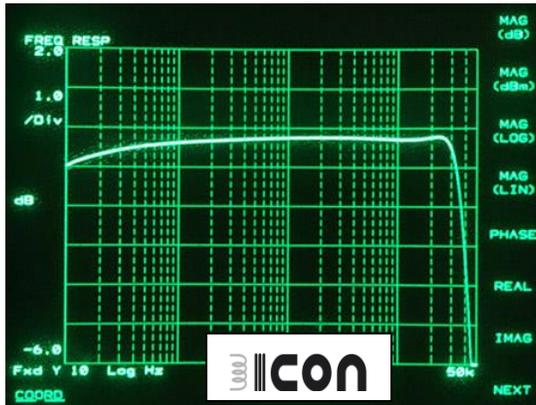
From 10Hz to 35,000Hz the frequency response is only -1dB deviation from 1KHz reference point. Source impedance is 12K ohm, load impedance is 10K ohm with a series primary connection.
