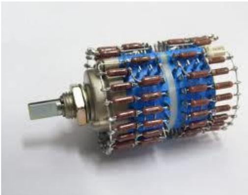
It requires the source to provide the power to drive the volume control's resistance which can result in currents as high as 2mA
